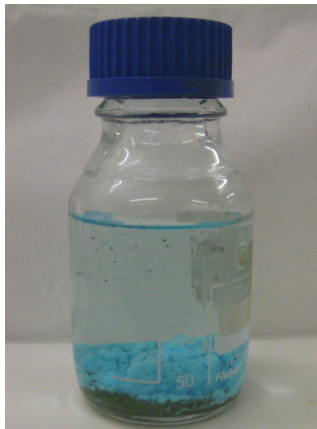
Fig. 1 Formation of green libethenite in the presence of original colloidal precipitate of blue basic copper phosphates
